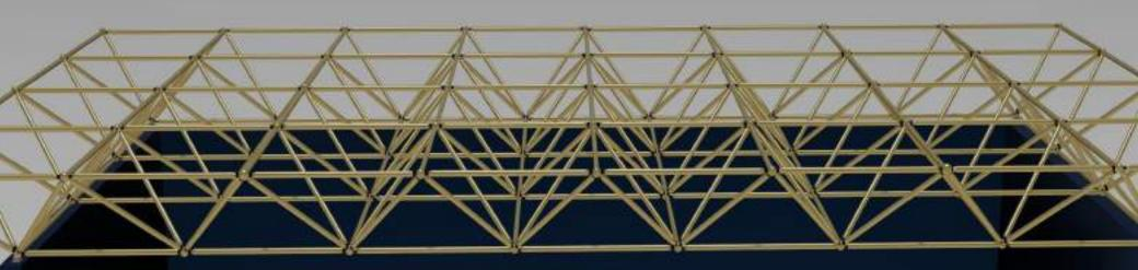
• Space frame is a rigid structure with truss-like composition that consists of several struts that are interlocked in a geometric pattern. one of the biggest advantages of a space structure is its strength, which allows for the creation of large areas with little to no internal supporting structures.
