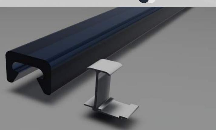
Polycarbonate snap on and aluminum hock connection that can be attached to the tabs on both sides of Megalux panels provide easy and safe installation. In this way, the system shows excellent water and air insulation performance and very good resistance against high roof and facade loads.
